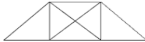
(b) Queen Post Roof Truss
