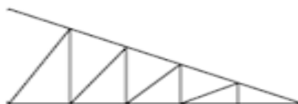
(k) North Light Roof Truss
