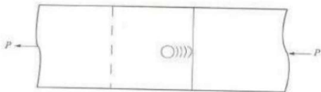
Crushing of plates.
